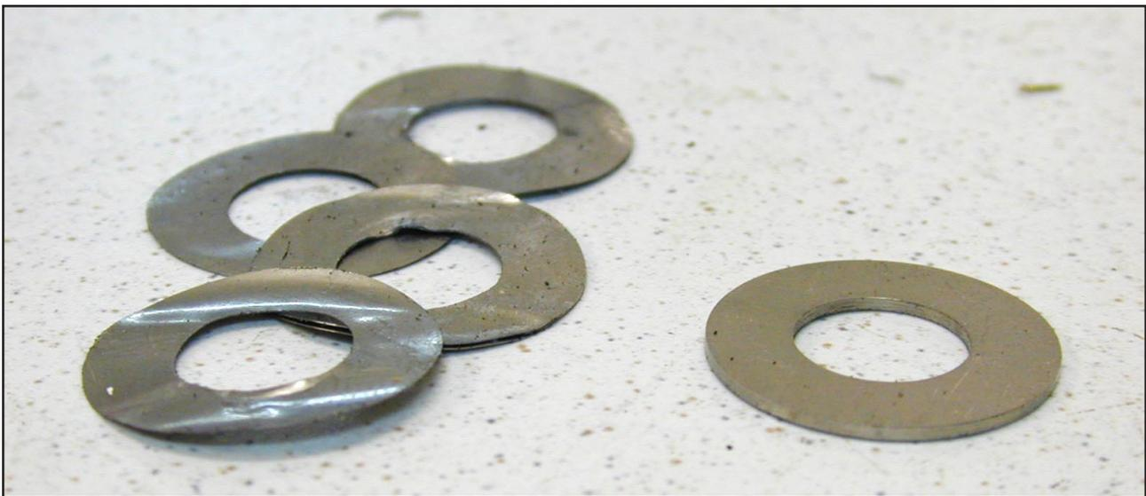
*A complete laminated shim is pictured on the left; on the right are individual layers that have been removed from another shim. Although the layers take a bit of a beating during the removal process, they could probably be straightened out with a flat hammer if necessary*
