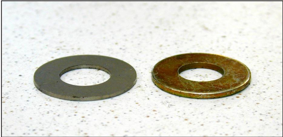
*Although at first glance there appears to be little difference between these two washers, in fact the one of the left is made up of no less than ten individual layers of extremely thin metal!*
