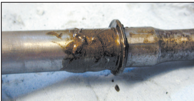
Once the snap ring and washer are installed on the shaft, thoroughly lubricate them with grease or anti-seize
