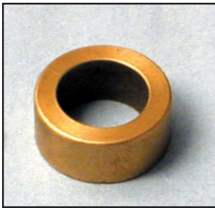
Dennis Quella has machined a new oillite bearing to replace the often-damaged nylon bushing in the bottom of the tube
