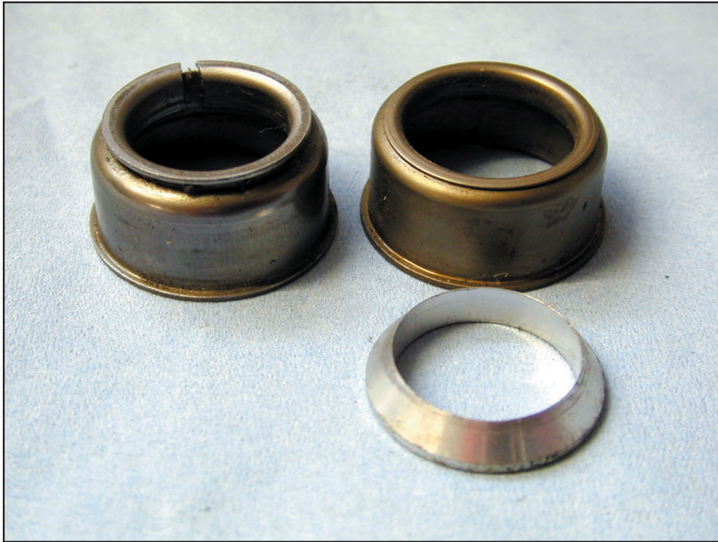
An original steering tube upper bearing on the left, with a new replacement bearing on the right. The machined aluminum centering spacer slides over the top of the steering shaft, and indexes on the curved radius of the bearing, centering the shaft perfectly
