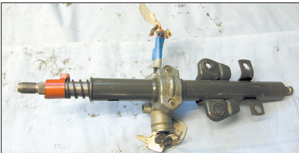
The overhauled and blueprinted steering column, ready for installation in the car
