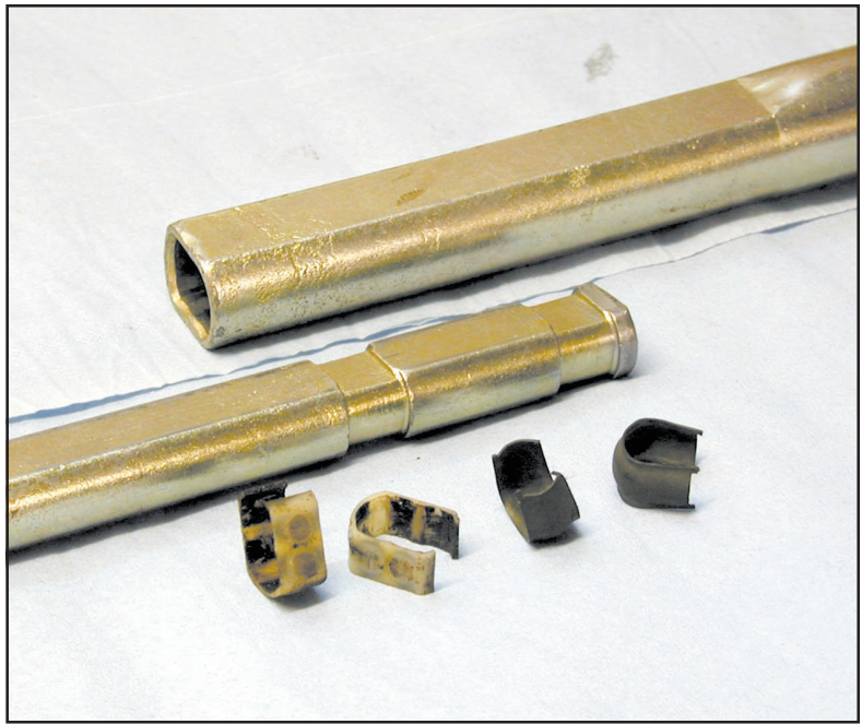
The male and female slider portions of the steering shaft system (these have been freshly cad-plated), along with the original nylon bushings (the two circular raised spots on each side are almost entirely worn away), and Wilkinson's stamped steel replacements
