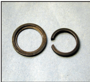
A snap ring positively engages a steel washer (which indexes on the snap ring); the other side of the washer rests against the bottom edge of the bearing
