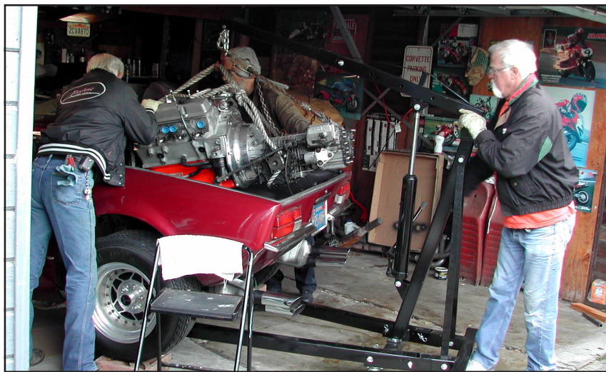
With skills borne of experience, Roger and Jim helped lower the engine/gear-box into the engine bay
