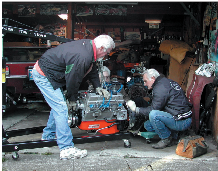
Jim carefully adjusted my throwout bearing with shims, for perfect operation
