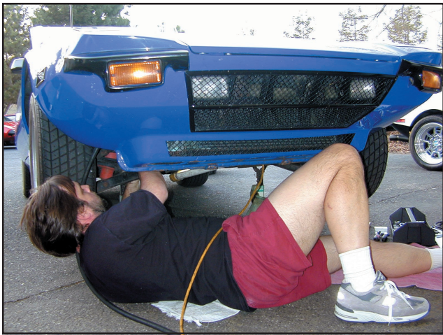
Marcus Smith adjusted his shocks, and installed factory-style spacers to alter his pre-L Pantera's steering geometry to the later, better L-model standard
