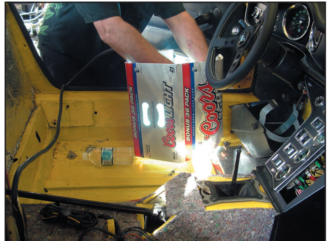
Mike Drew and Kirk Evans drove Mike's Pantera over 200 miles on the way to the party; later Kirk thought 'inside the box' as he welded new seat rail mounting nuts to the custom floorboards
