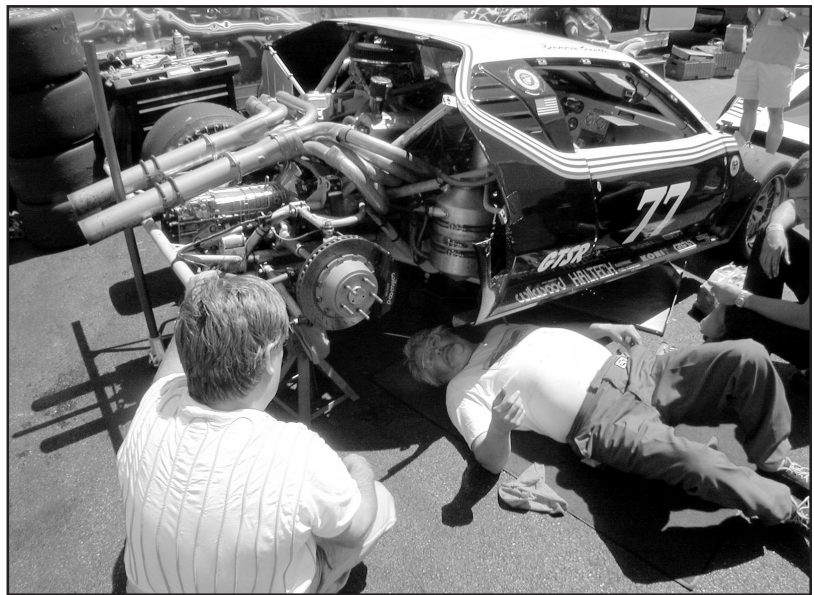
Dennis Quella struggled with an oil system problem all weekend. His oil pump would fill the valve covers with oil, blowing the breather off and coating the engine bay with oil. The only solution was to slow down, which is definitely not his style!
