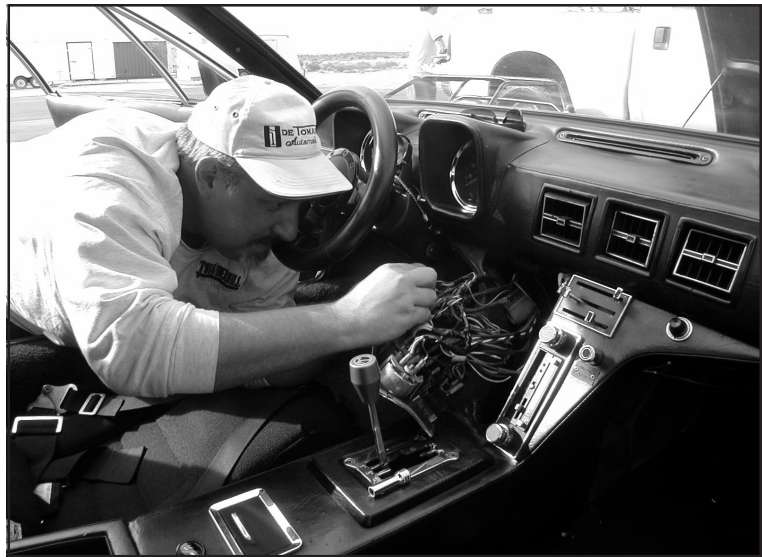
"Sparky Mark" McWhinney tore into his instrument console to track down and fix an electrical fire, caused by poor ammeter connections
