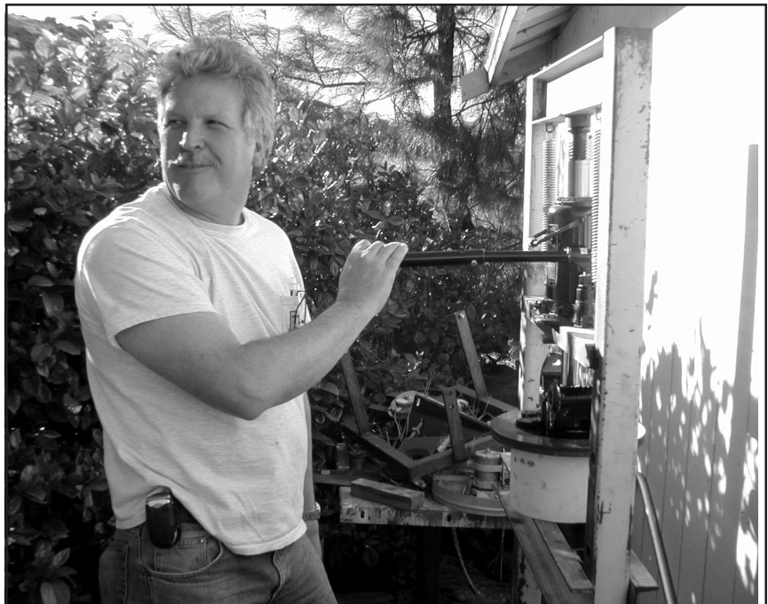
Larry Stock mans the press, removing perfectly good wheel bearings and replacing them with another set of perfectly good wheel bearings. New axle, anyone?
