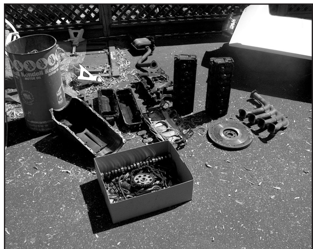
The pile of parts heading for the trash includes the cylinder heads, cam, flywheel, exhaust, and oil pan.
