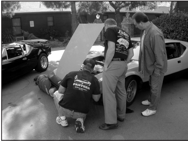
Several members of the tech crew attended to Diane's water leak, which was caused by a loose hose clamp
