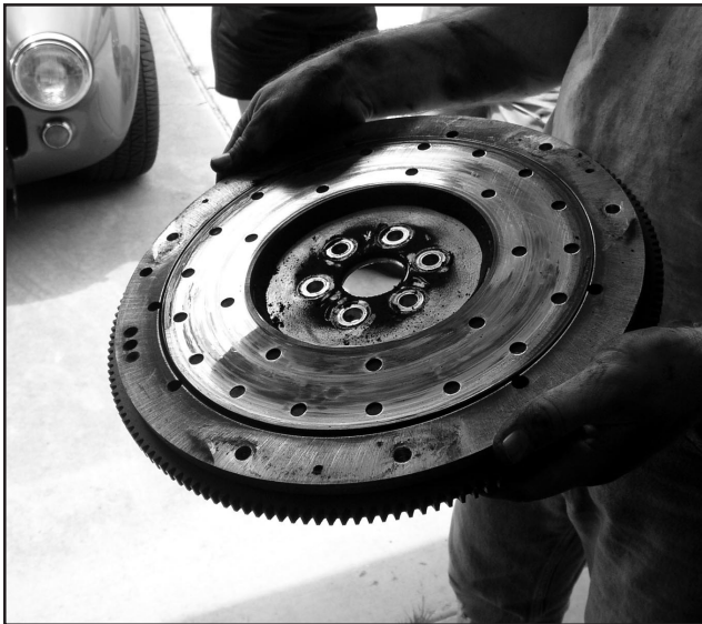
The sexy aluminum flywheel was badly scored by the rivets on the clutch disc, and had to be resurfaced
