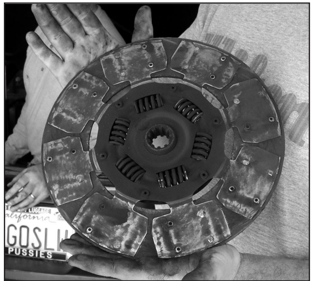
The clutch disc had absolutely zero friction material left!
