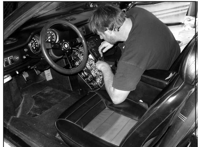
Marcus found a rat's nest of wiring under the dash, and isolated several potential electrical fire sources!
