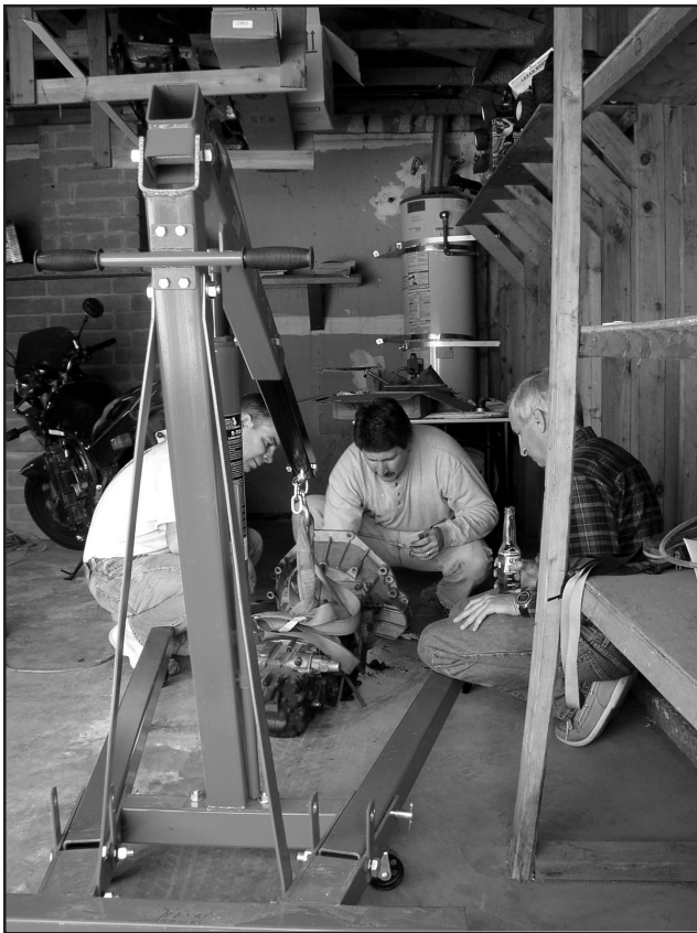
With the gearbox out, changing the demolished throwout bearing was the next task
