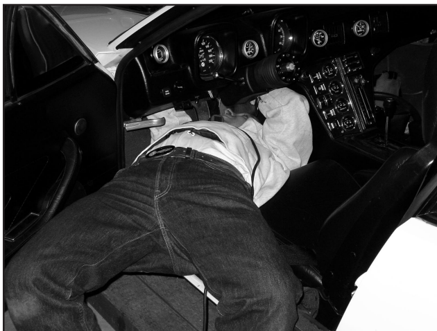
Later that night, Mike spent a good half hour on his back underneath Greg's dashboard, adjusting the clutch linkage to ensure proper pedal height and full clutch throw
