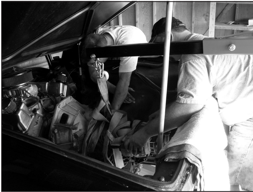
The gearbox was carefully lowered back into position
