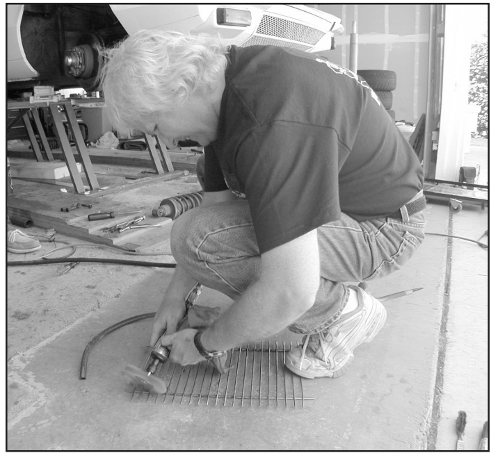
Rick "does the dishes" with a wire wheel on a die grinder!
