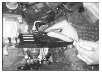
This clutch slave cylinder bleed screw proved to be especially difficult. Fortunately I had a spare clutch slave cylinder lying around, and the bleed screw from that one worked great
